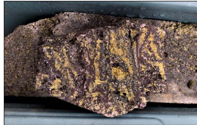
Hematite - specular hematite – magnetite – quartz – chalcopyrite at 423.5m (cut surface).
