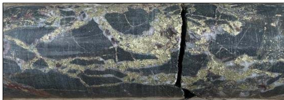
Chalcopyrite+quartz-filled fractures in chlorite+quartz-altered microdiorite. 390.6m.
