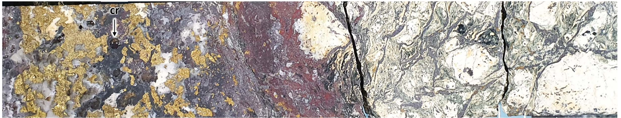
Photograph of drill-core from SMD159 at about 553m and core box (550.9m to 553.9m) in the hangingwall of the Cayley Lode, showing the replacement of a wedge of serpentinized ultramafic (right) by massive chalcopyrite-hematite-magnetite-quartz-chlorite (left) with crystals of chromite ('cr'). The assay result for the interval 552.7m to 553.3m indicates: Au – 0.1 ppm, Ag – 21 ppm, As – 9 ppm, Cr – 1500 ppm, Cu – 5.62%, Fe – 19.3%, Mo – 1 ppm, Ni – 524 ppm, S – 5.25% and Zn – 39 ppm.
