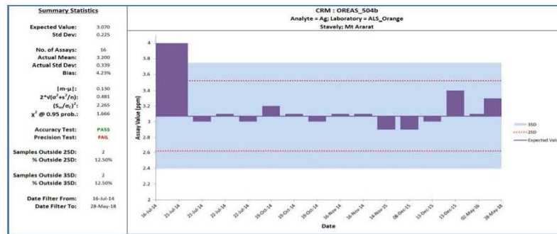
Figure 3-1 OREAS_501b Silver; Negative bias -11.63% (precision test fail)
