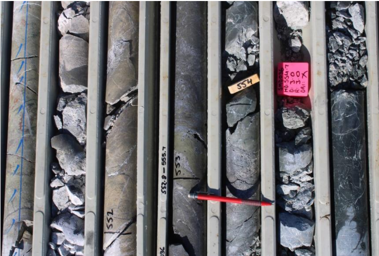
Photo 3 Sulphide-rich structure with sericite alteration selvage which plots close to the project of the NS fault on the cross section, DDH SMD036, 553-5m.
