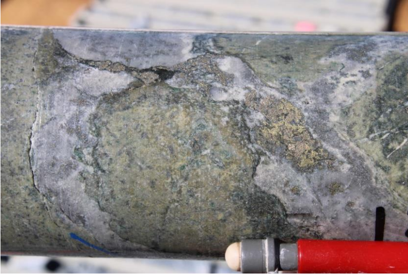
Photo 18 Porphyry vein-dykes with pyrite-chalcopyrite, Stavely DDH SMD036, 234m.
