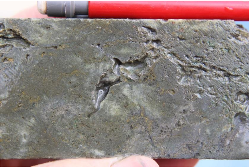
Photo 21 Low sulphidation quartz-pyrite vein overprinted by vuggy residual silica, DDH SNDD1, 163.2m.
