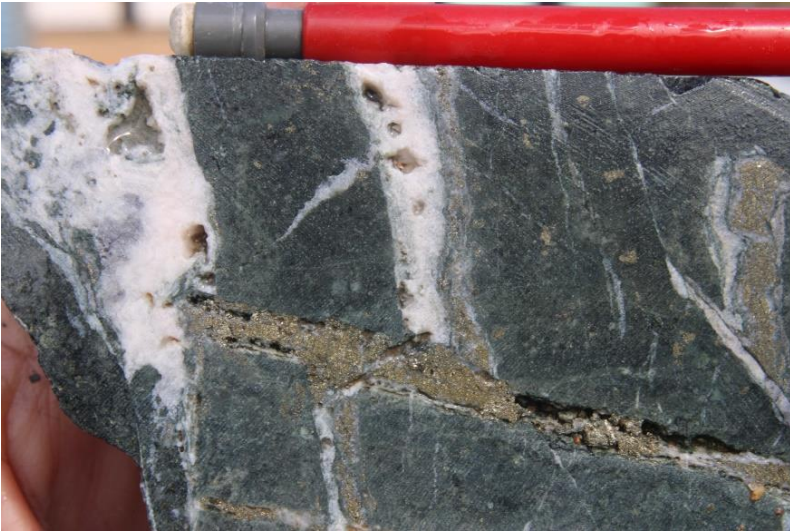
Photo 12 Low sulphidation Au mineralisation developed by the mixing of a rising pregnant magmatic fluid which deposited quartz-pyrite, with bicarbonate waters evidenced by rhodochrosite, DDH SMD026, 243.5m, 0.56 g/t Au.
