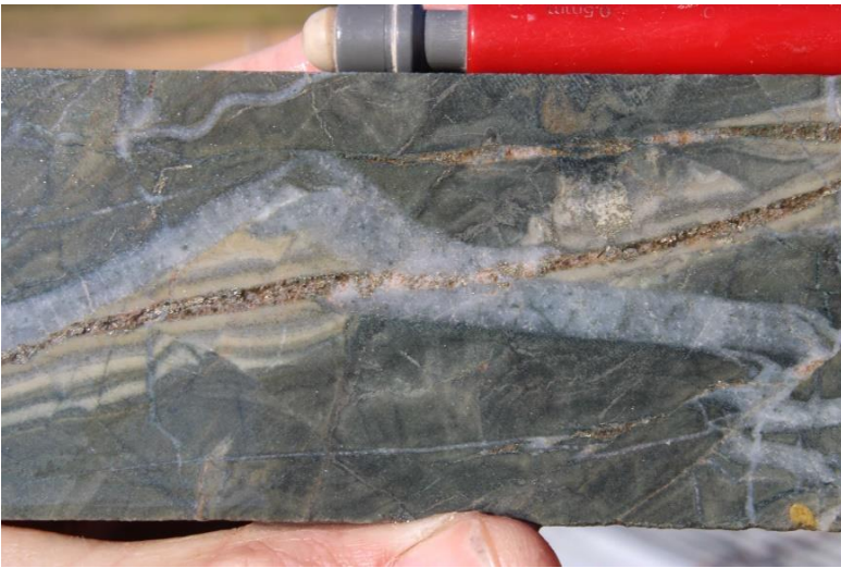
Photo 10 Porphyry style D vein with sericite selvage cuts A vein, DDH SMD026, 599.1m.
