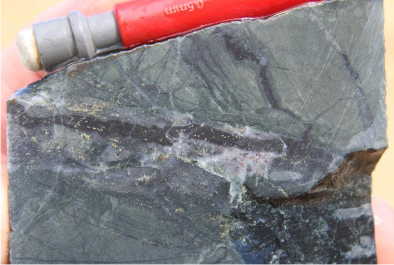
Photo 27 Transitional A-M vein of quartz and magnetite but without a laminated form, DDH SMD24 437m.
