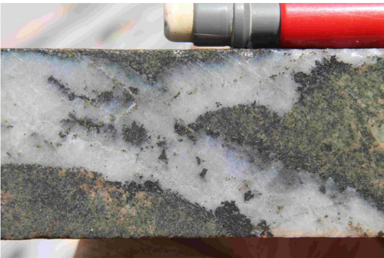
Photo 29 AM vein from Ridgeway, NSW, within the mineralised interval, DDH NC498, 701.5m.
