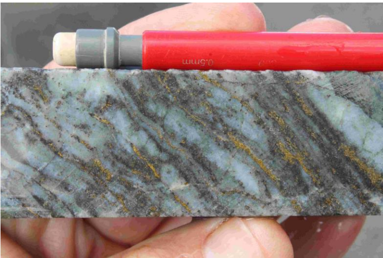
Photo 28 M vein from Copper Hill NSW showing chalcopyrite deposition within partings between quartz-magnetite laminations, DDH64, 120.2m, 15.2 g/t Au & 3.03% Cu.
