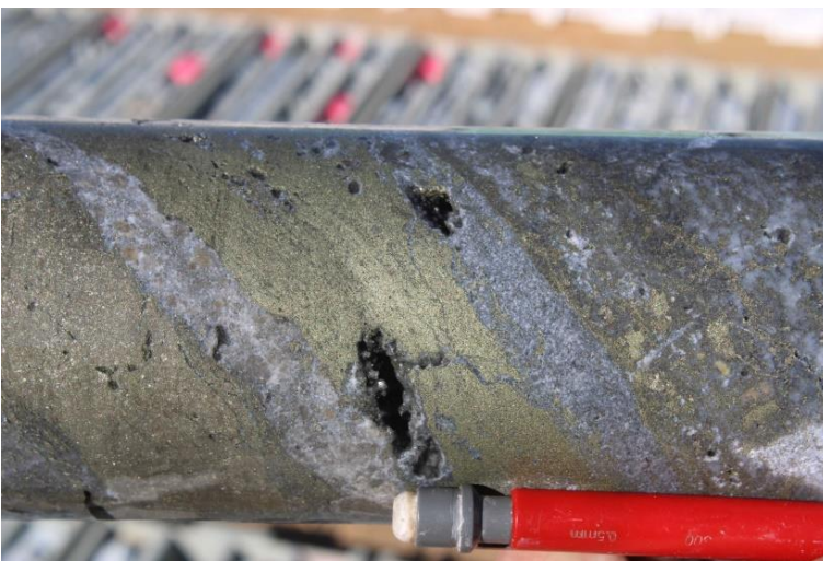
Photo 4 Close up of the sulphide-filled structure in photo 3 showing banded pyrite and chalcopyrite interpreted as a fault-fill D vein, DDH SMD036, 553m.
