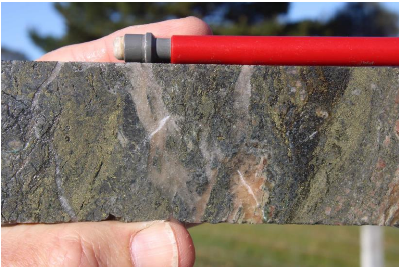
Photo 26 D vein with pyrite-chalcopyrite and anhydrite, DDH26, 628.5m, 0.8 g/t Au & 2.3% Cu.G
