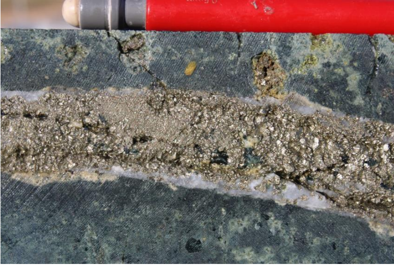
Photo 9 Low sulphidation epithermal quartz-pyrite vein with prograde chlorite alteration selvage cuts epidote wall rock alteration, DDH SMD026, 198m.
