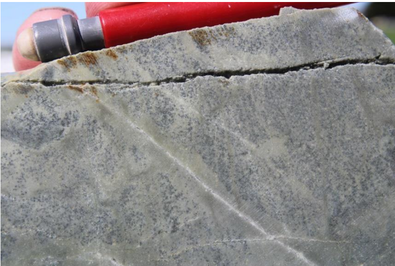
Photo 25 Disseminated chalcopyrite is remobilised from the sericite selvages to fractures, DDH SMD031, 116m.
