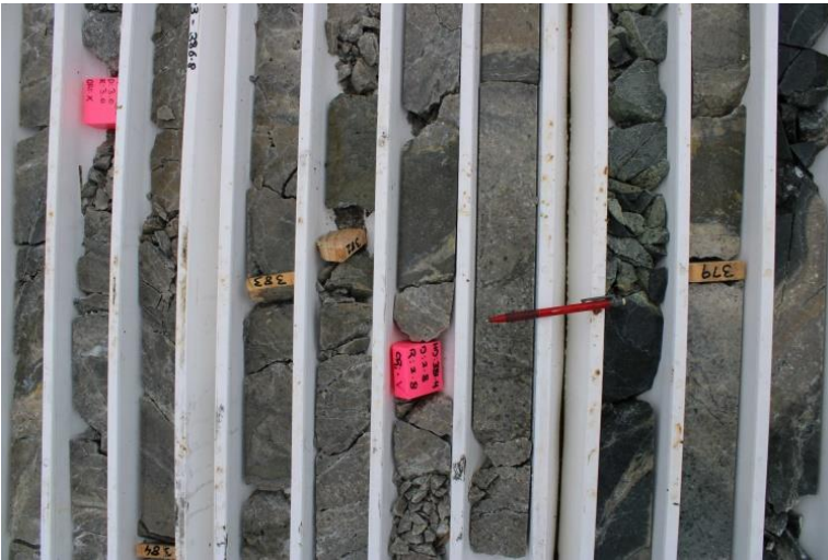
Photo 16 Broad phyllic alteration adjacent to D veins, DDH SMD016, 379m.
