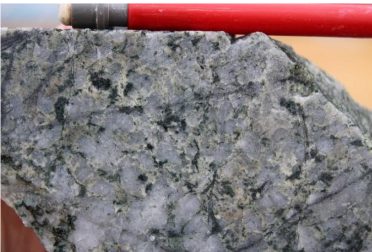
Photo 35 Spotty quartz typical of the uppermost portion of a porphyry intrusion, DDH SMD023, 177.5m.
