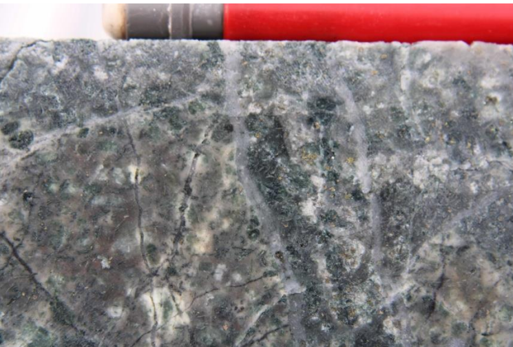
Photo 8 K-feldspar altered intrusion cut by quartz-actinolite veins, DDH SMD017, 478.6m.
