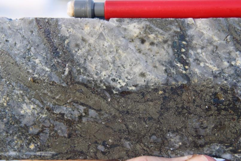
Photo 21 D vein dominated by pyrite and bornite, DDH SMD015, 197.5m.
