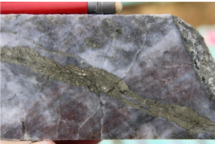
Photo 32 Laminated quartz-magnetite vein cut by a pyrite D vein with alteration of the magnetite to haematite, DDH23, 135.9m.
