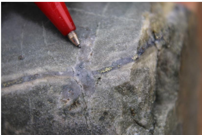
Photo 18 Quartz-pyrite-chalcopyrite-molybdenite, DDH SMD024, 285.9m.
