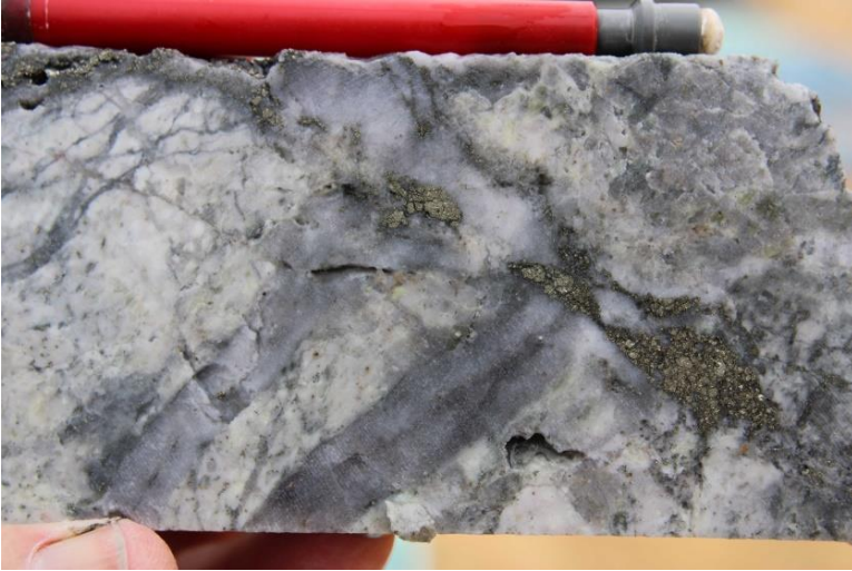
Photo 30 A-M veins cut by a pyrite D vein, DDH SMD023, 156.5m.
