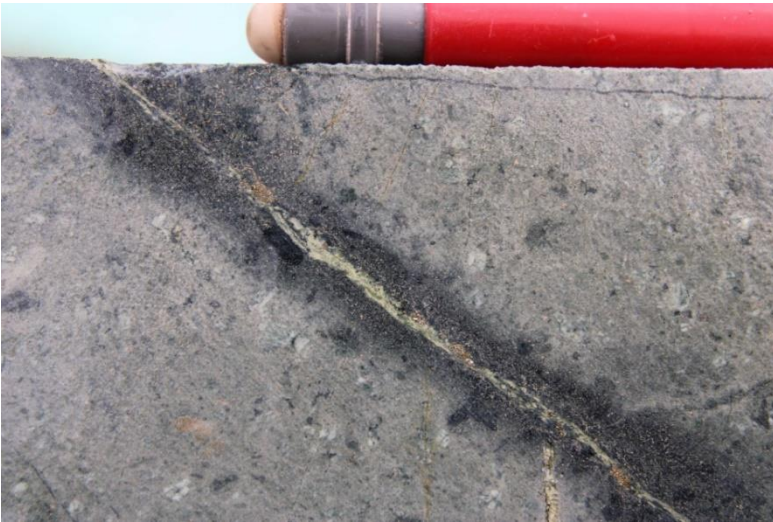
Photo 10 Pervasive sericite cut by epidote-chlorite vein, DDH SMD013, 161.9m.
