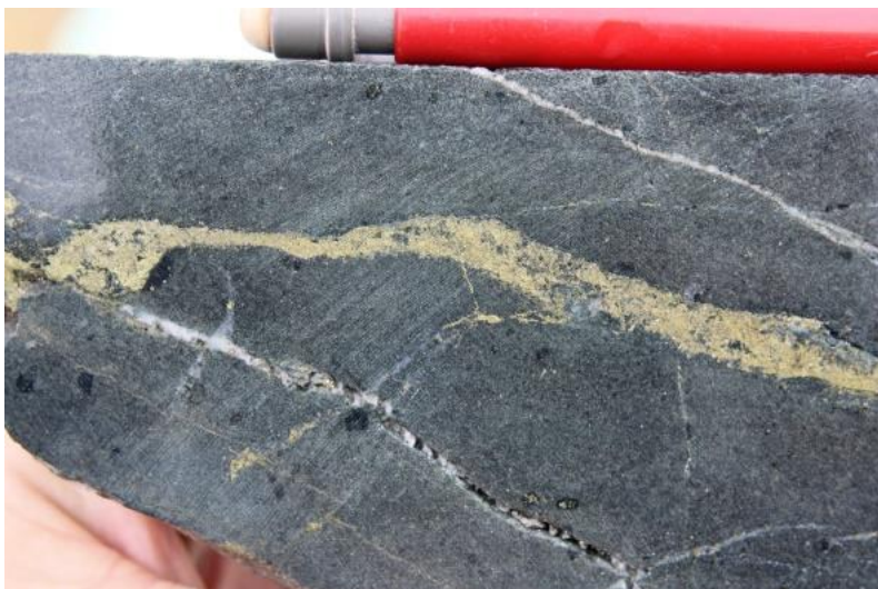
Photo 20 Porphyry style chalcopyrite-dominant C vein cuts unaltered andesite, DDH SMD014, 328.3m.
