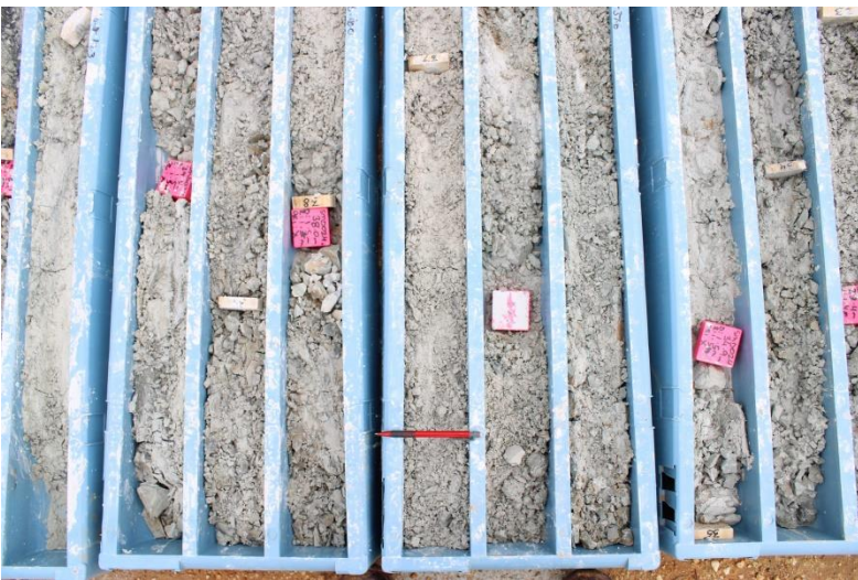
Photo 11 Clay as argillic alteration overlying phyllic alteration, DDH SMD24, 38m.
