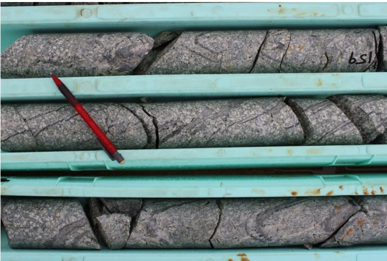
Photo 13 Porphyry with pervasive phyllic alteration with quartz veins, DDH SMD020, 158m.
