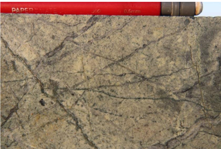
Photo 4 Quartz-magnetite veins cut pervasive sericite, DDH SMD014, 216.8m.
