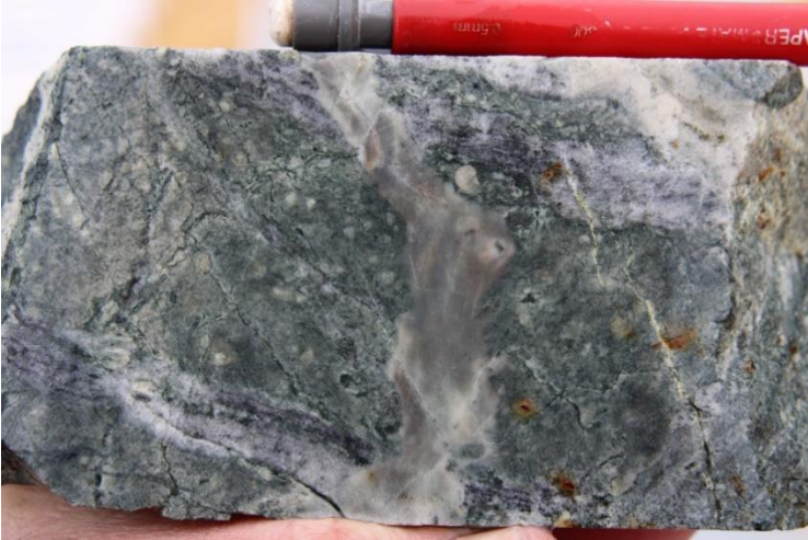
Photo 33 Aplite dyke cuts quartz-magnetite veins with actinolite alteration, DDH SMD017, 424.8m.
