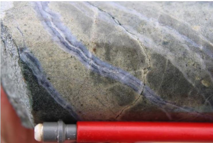
Photo 25 The uppermost M veins in drill hole 24 contains watery chalcedonic to opaline quartz typical of a low temperature of formation, DDH SMD024, 339.5m.
