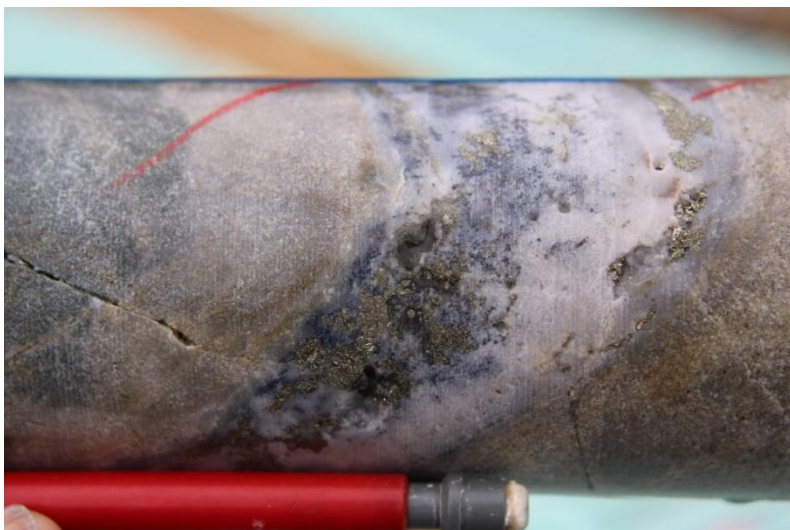
Photo 19 Quartz-pyrite-molybdenite D vein with sericite selvage, DDH SMD024, 332.1m.
