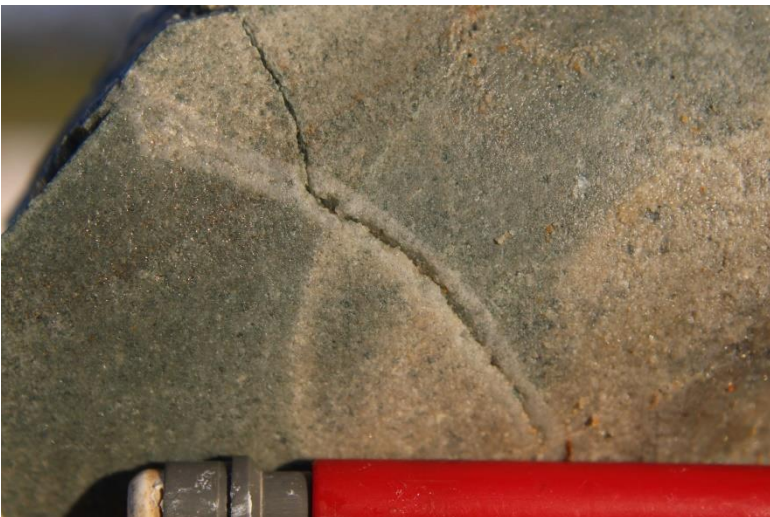
Photo 14 Chlorite-sericite alteration at the margin of pervasive phyllic alteration cut by a B vein, DDH SMD014, 39m.
