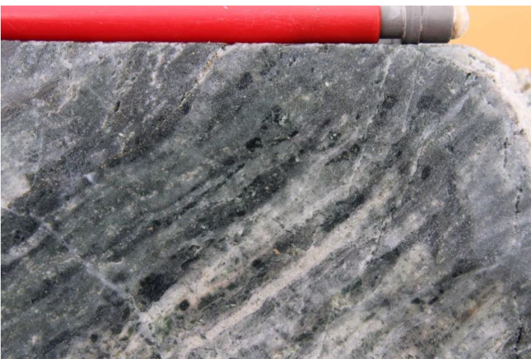
Photo 29 Laminated quartz-magnetite vein with actinolite alteration, DDH SMD017, 443.6m.
