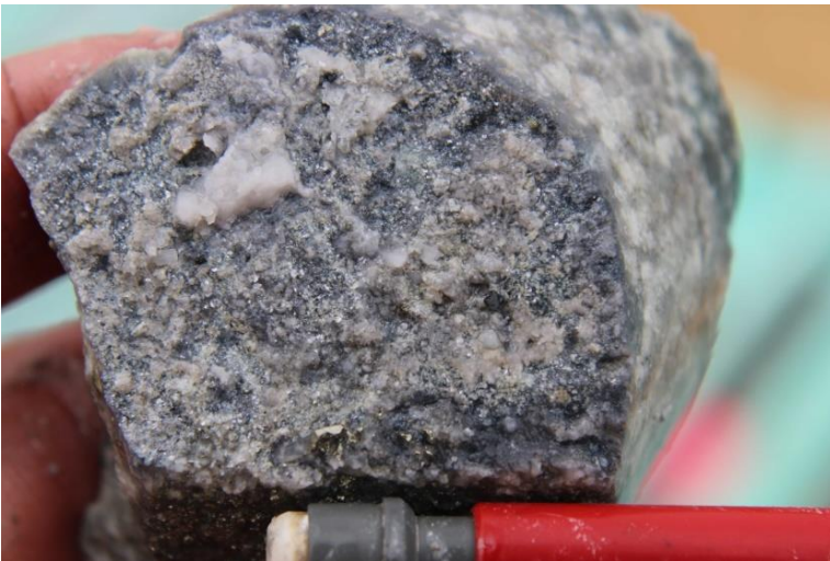
Photo 17 Quartz-molybdenite on a fracture, DDH SMD024, 293.7m.
