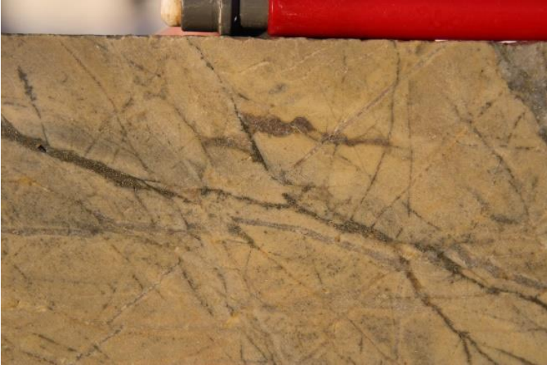
Photo 12 Pervasive sericite with fracture controlled pyrite, DDH SMD014, 166.4m.
