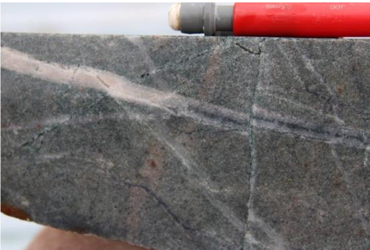
Photo 34 Aplite dyke cut by A-M veins, DDH SMD017, 446.4m.
