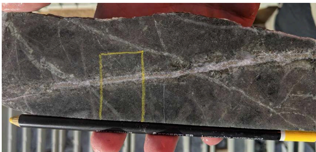
Fig. 25: Drill core sample of possible andesitic or microdioritic rock with initial biotite alteration, cut by early quartz-rich veins and by a later, major vein of carbonate and pyrite. Retrograde propylitic alteration, forming chlorite-sericite-carbonate is overprinting biotite alteration and is commonly vein-controlled.
