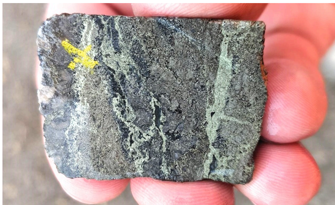
Fig. 1: Drill core sample of semi-massive, weakly banded sulphides, with zones rich in pyrite and pale grey quartz that are invaded by irregular to veinlike chalcopyrite aggregates.
