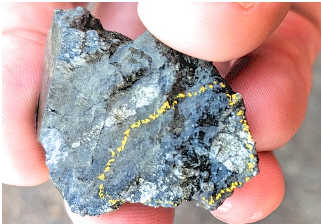
Fig. 4: Drill core sample of sulphides-rich aggregates (dark) that are intercalated with and enclose fragments of, fine grained quartz (-sericite) rock. Sulphides are dominated by pyrite, with minor chalcocite and other Cu sulphide phases.
