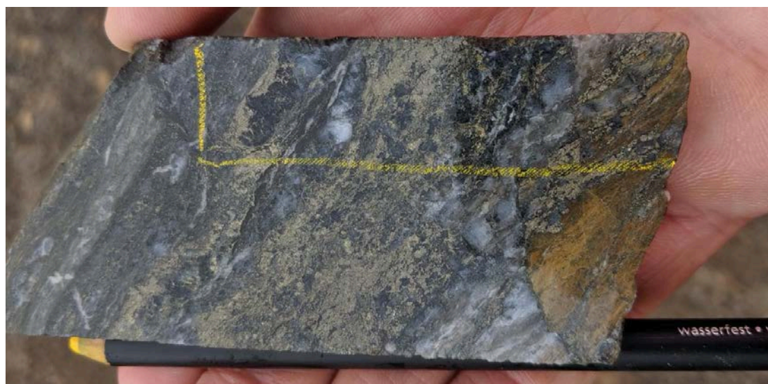
Fig. 20: Drill core sample of sheared host rock (possibly sandstone) with intercalated quartz- and sericite-rich bands, overprinted by largely co-planar quartz-sulphide veining. Quartz and abundant pyrite are overprinted by paragenetically later chalcopyrite.
