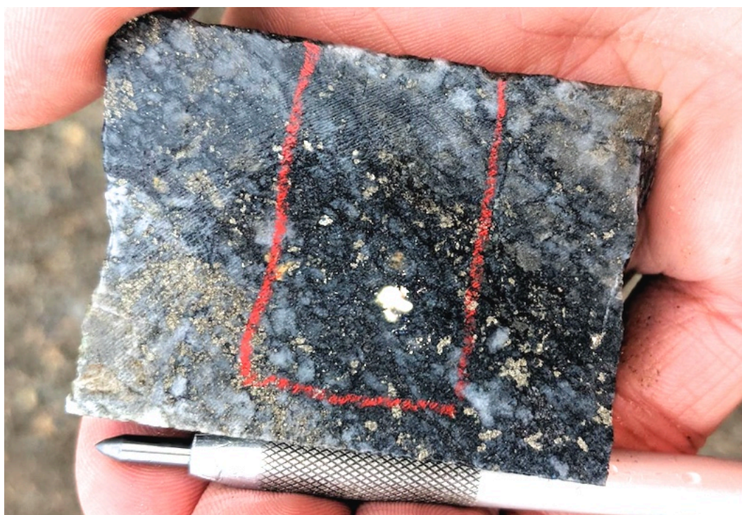
Fig. 11: Drill core sample of slightly banded quartz-sulphide rock. Disseminations and aggregates of pyrite are evident in quartz, with the dark grey zone containing considerable Cu sulphides that include bornite, enargite, chalcocite and digenite.
