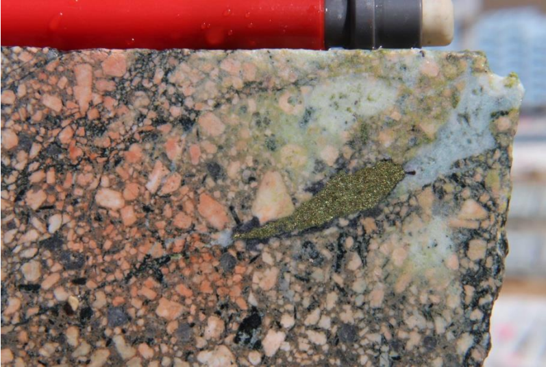
Photo 23 Mt Stavely prospect coarse grained dacite with chalcopyrite rimmed by bornite with epidote-quartz alteration, DDH MSD001, 406m.
