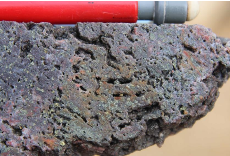
Photo 6 Vuggy residual silica formed as part of the advanced argillic alteration associated with an enargite-pyrite bearing D vein, DDH SNDD1, 100.2 m.
