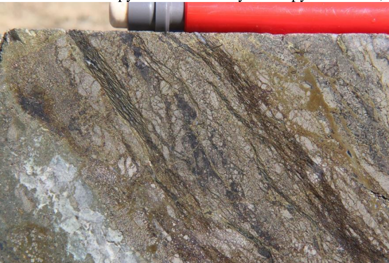
Photo 13 Massive pyrite D vein cut by chalcopyrite followed by bornite, DDH SMD016, 336.3 m.
