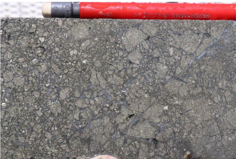
Photo 4 Close up of the massive pyrite in photo 3 showing minor quartz, DDH SMD044, 324.9 m.
