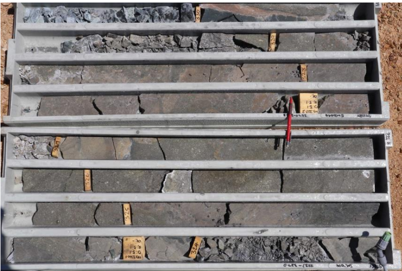
Photo 3 A several metre wide drill intercept of massive pyrite with sericite altered wall rock, DDH SMD044, 324.9 m.
