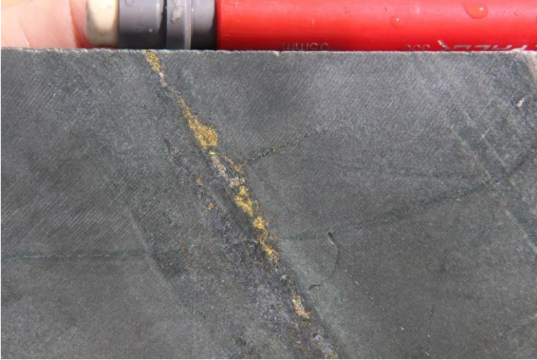
Photo 20 Chalcopyrite on a reactivated bedding plane, DDH SMD029, 831.1 m.
