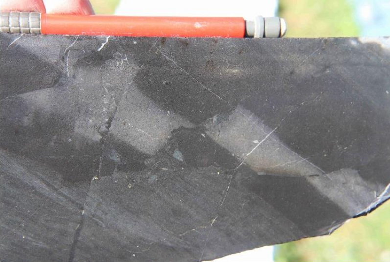
Photo 22 Disrupted bedding in wall rocks adjacent to an Alfa 1 breccia pipe, DDH SMD105, 307.8m.
