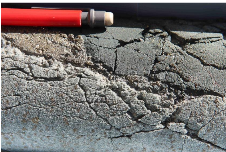
Photo 20 Contact between two Alfa 1 breccia bodies which has been exploited by a D vein, DDH SMD131, 80m.
