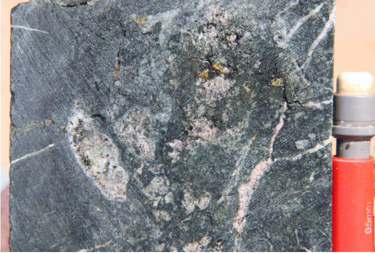
Photo 43 Fluidised portion of Alfa 2 breccia reaction rimmed quartz as well as chalcopyrite clasts, DDH SMD44, 675.6m, 3720ppm Cu.
