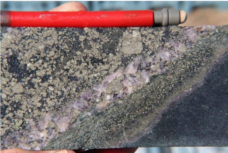
Photo 69 G vein characterised by magnetite-haematite-pyrite-anhydrite-pyrite ± chalcopyrite without the significant sericite selvage which characterised D veins, DDH SMD117, 723.1m.
