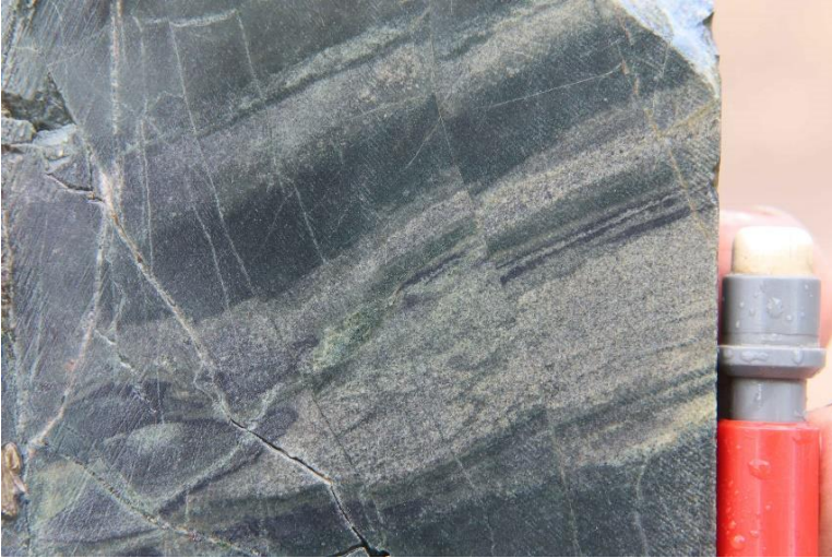
Photo 61 Possible Kfeldspar alteration of a permeable reactive band in the volcanosedimentary sequence, DDH SMD047, 609.5m.
