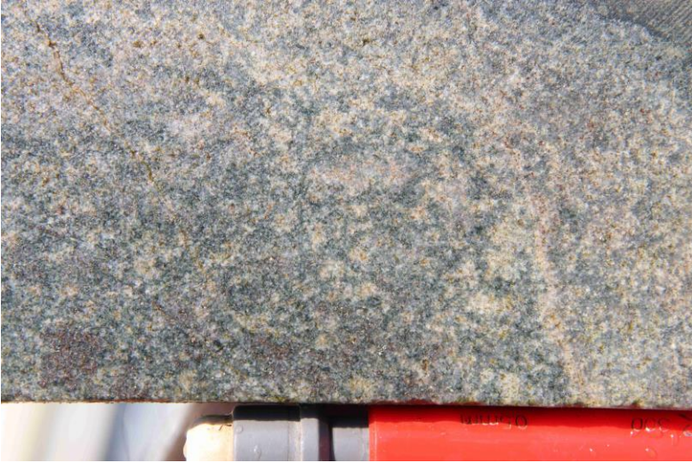
Photo 13 P2 intrusion showing pink ?albite alteration along with magnetite and chalcopyrite, DDH SMD44, 604.1m, 2600ppm Cu.
