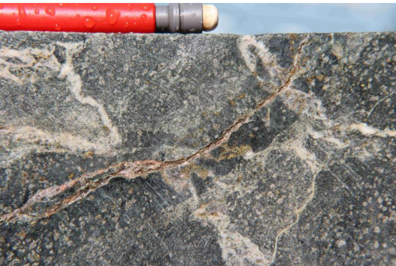
Photo 39 Green fluidised breccia dyke with chalcopyrite in Alfa 2breccia, DDH SMD44, 689.7m, 2970ppm Cu.
