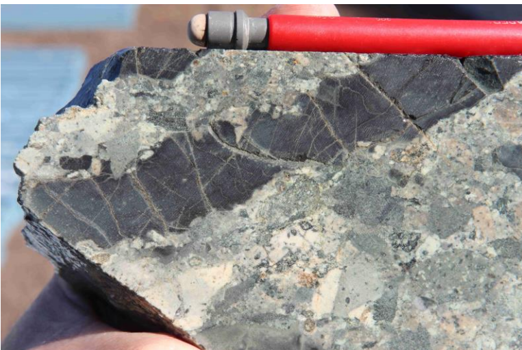
Photo 9 Ragged and embayed fine grained black felsite clast in Alfa 2 breccia, DDH SMD31, 100.8m.
