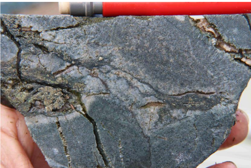
Photo 36 DDH Actinolite-pyrite fill fracture and clast or bleb of sulphide within Alfa 2 breccia, DDH SMD44, 606.9m, 9530ppm Cu.
