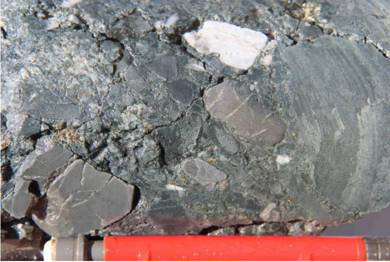
Photo 4 Alfa 1 breccia with pink felsite clasts, a pale silicified ultramafic clast and bedded tuff, DDH SMD131, 76.7m.
