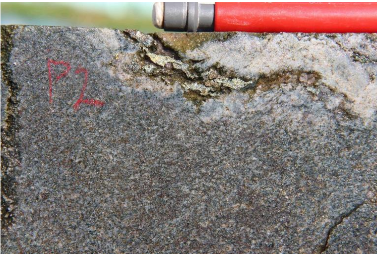
Photo 14 P2 intrusion with disseminated magnetite-chalcopyrite and a ?albite-chalcopyrite vein, DDH SMD44, 657.3m, 1210ppm Cu.
