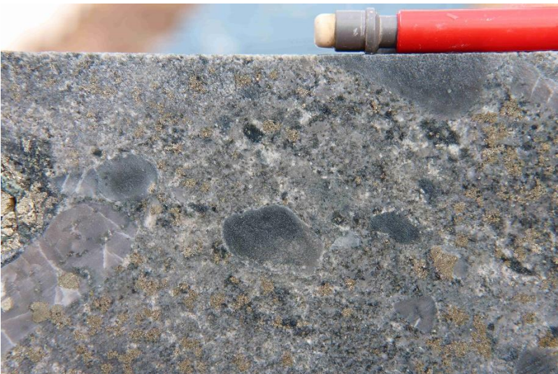
Photo 3 Alfa 1 breccia formed by a mix of altered comminuted rock clasts, including pink felsite, probable microdiorite with the addition of hydrothermal pyrite, DDH SMD146, 178.1m.
