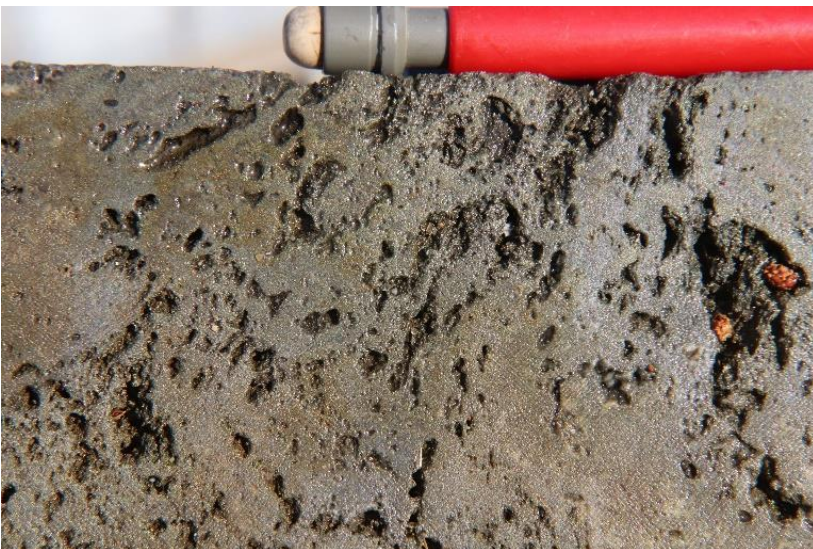
Photo 11 Pyrite, bornite, chalcocite with vuggy silica, DDH SMD51, 149.2, 12.2% Cu & 3.33 g/t Au.
