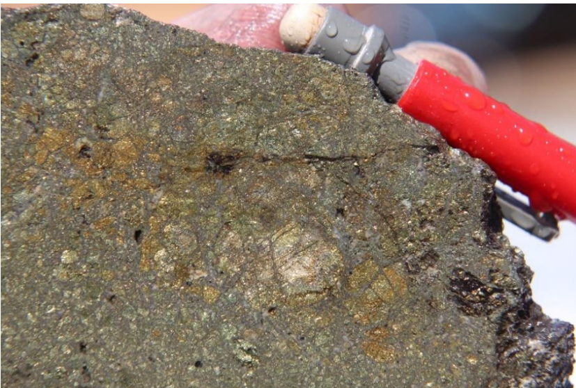
Photo 5 Chalcopyrite overgrows pyrite, DDH SMD50, 89.9m, 1.28% Cu & 0.64 g/t Au.
