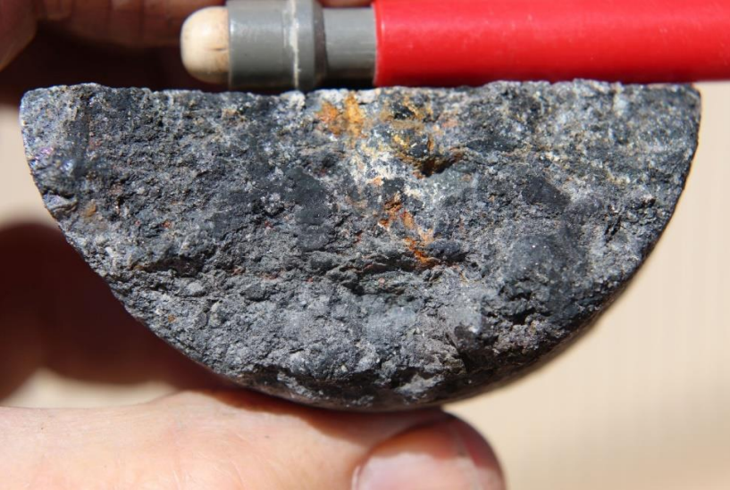
Photo 12 Fracture with supergene chalcocite which yielded a hand held XRF assay of 55% Cu & 0.5% Ag, SMD50, 65.5m.
