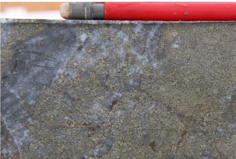
Photo 4 Quartz-pyrite D vein, DDH SMD54, 90m, 0.23% Cu & 0.05 g/t Au.
