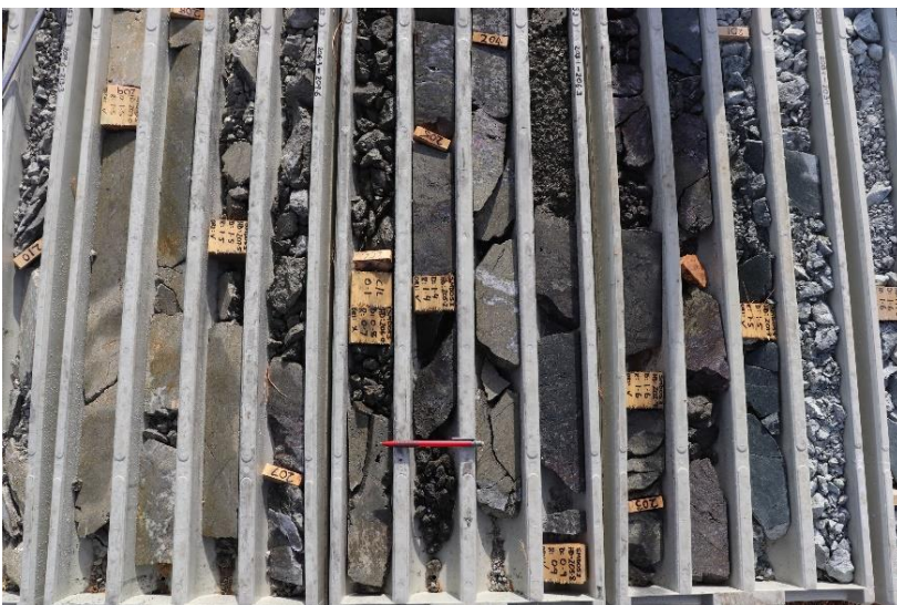
Photo 2 View of the Sulphide Lode in DDH SMD53 200-210 m grading from outer D vein pyrite to central Cu sulphides (photo 10).
