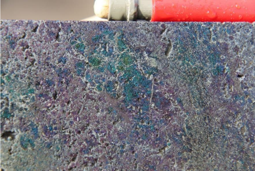
Photo 9 Massive bornite with later chalcocite DDH SMD50, 82.7m, 21.6% Cu & 3.8g/t Au.
