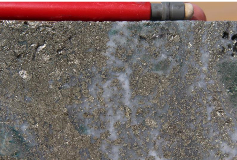
Photo 3 Typical quartz-pyrite D vein characterised by coarse crystalline pyrite and white quartz, DDH STRC19D, 148m.
