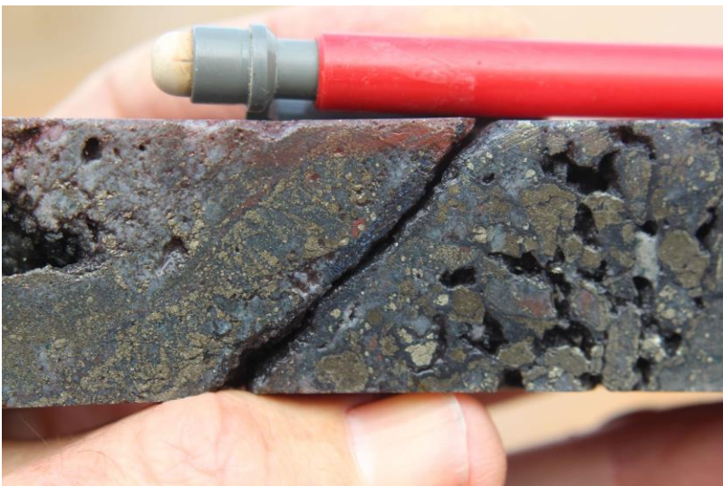
Photo 7 Quartz-pyrite vein (left) cut by chalcocite matrix breccia (right) with pyrite clasts, DDH STRC19D, 151.4m.
