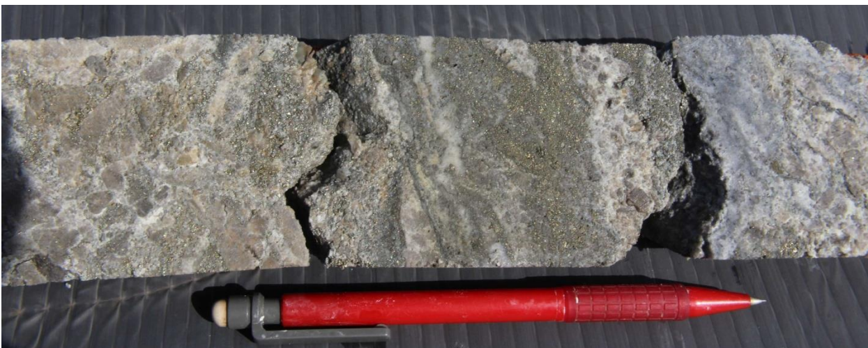
Photo 1 Porphyry D vein which comprises the early Mo-rich D vein at the margins and later cross-cutting central pyrite-dominant D vein in the centre, DDHSM6, 173.7m.
