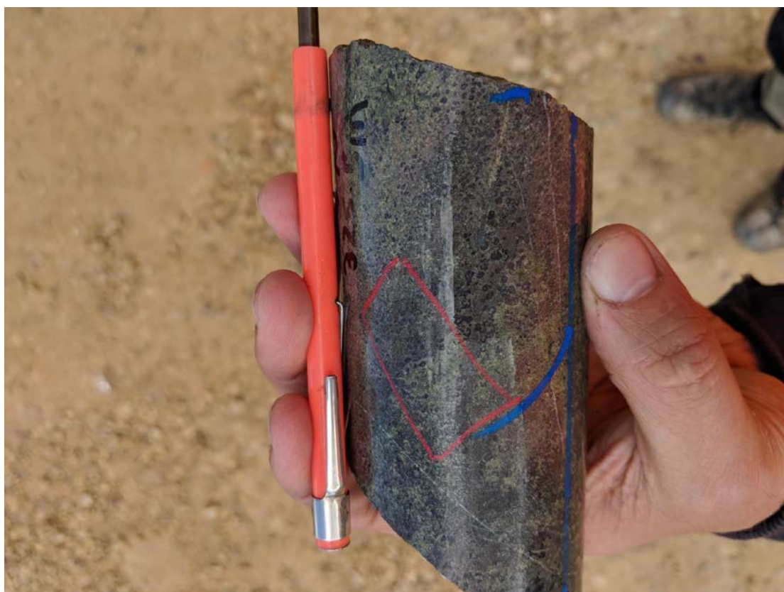
Fig. 22: Drill core sample of "skarn-like" rock derived by metamorphism and probable metasomatism of an originally amygdaloidal basalt. There is an initial assemblage of garnet-plagioclase-quartz, overprinted by epidote, and subsequently by retrograde chlorite and carbonate.
