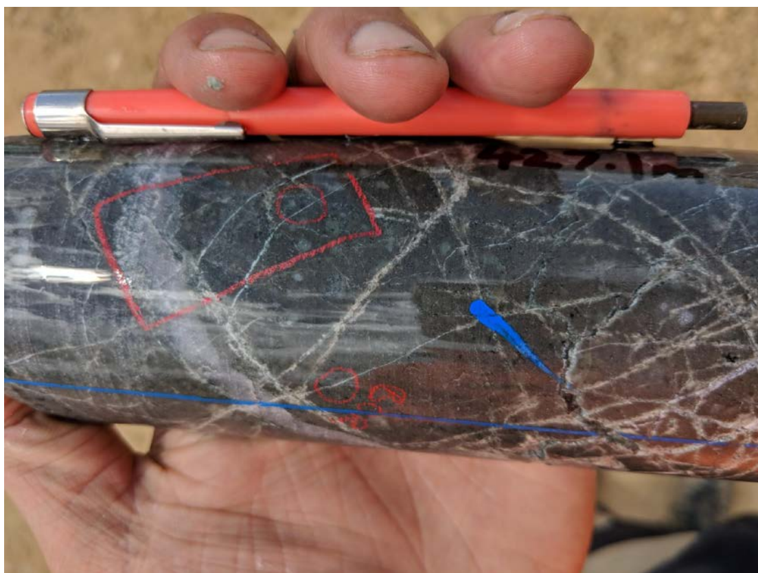
Fig. 25: Drill core sample of altered porphyritic quartz andesite that has pervasive propylitic alteration, with early quartz-rich veining cut by later thin carbonate-chlorite veins.
