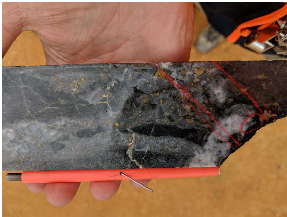
Fig. 1: Drill core sample showing paler grey quartz (-chalcopyrite-pyrite) veining in dark grey-green, intensely altered host rock (probably originally basaltic).
