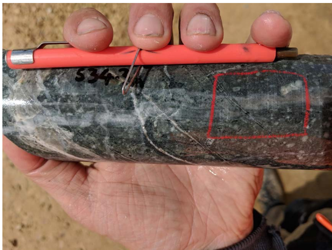
Fig. 16: Drill core sample of dark grey-green altered porphyritic andesite, with early veining by pale grey quartz and later veining by carbonate-rich aggregates (paler grey to white) that also contain quartz, pyrite and chalcopyrite.
