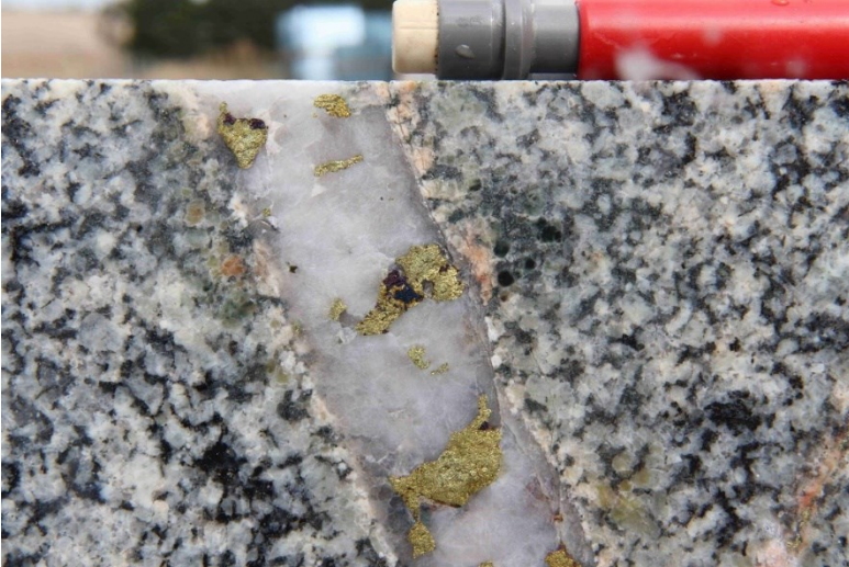
Photo 22 Toora West equigranular diorite cut by massive A-like vein with chalcopyrite-bornite, STWD7, 467.5m, 0.15% Cu.
