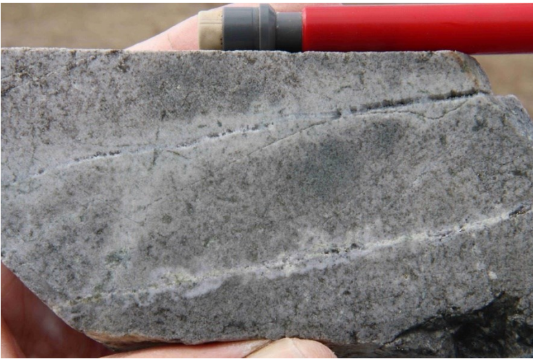
Photo 12 Toora West microdiorite with strong pervasive silica-sericite-pyrite (phyllic alteration), more intense adjacent to B vein and fractures, SMTD7, 66.5m.
