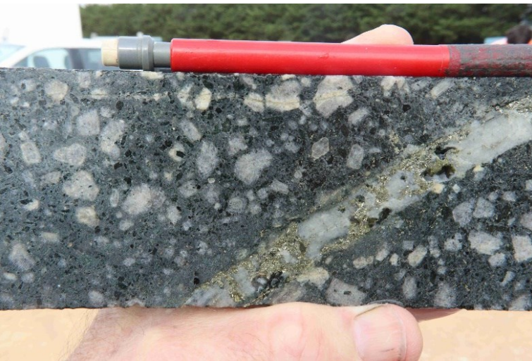
Photo 18 Toora West hornblende diorite porphyry cut by quartz-pyrite-chalcopyrite, STMD6, 69.7m.
