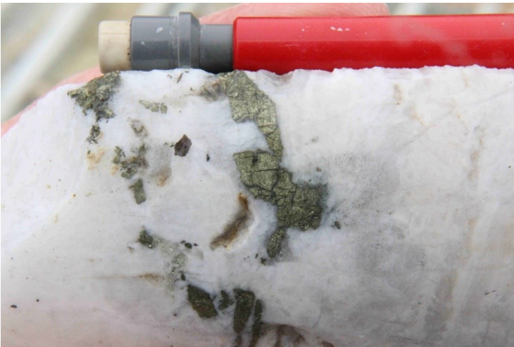
Photo 16 Toora West quartz vein with coarse pyrite-chalcopyrite and possible fracture fill chalcocite, STWD5, 274.4m, 60cm @ 4.27g/t Au, 2.3g/t Ag & 0.3% Cu.
