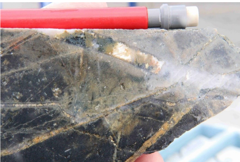
Photo 22 Toora West basalt cut by quartz-carbonate-pyrite-chalcopyrite actinolite vein, STWD7, 187.1m, 0.13% Cu.
