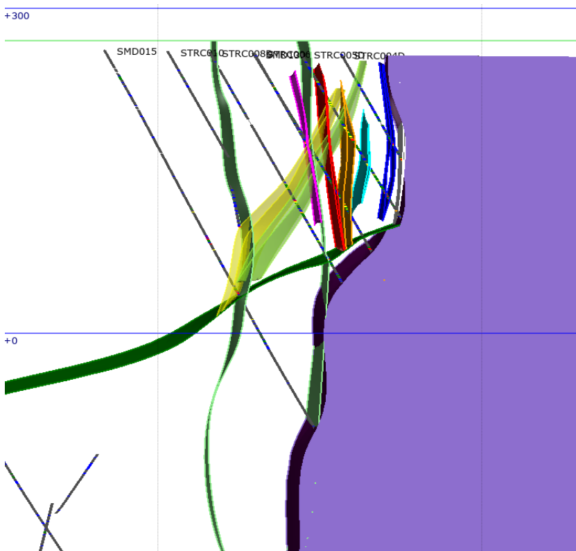
Figure 5 section 1, shown in figure 3 as the most northwesterly of this series of cross sections, is characterised by a steep-dipping set of Cayley Lodes developed in a negative flower structure configuration which terminates at the LAS, here interpreted as pre-mineral. The flower structure would normally be linked to the underlying steep-dipping Stavely Volcanics-ultramafic contact. The lack of offset on the vertically attenuated microdiorite suggests an emplacement after offset of the volcanic-ultramafic contact and probably prior to lode emplacement.
