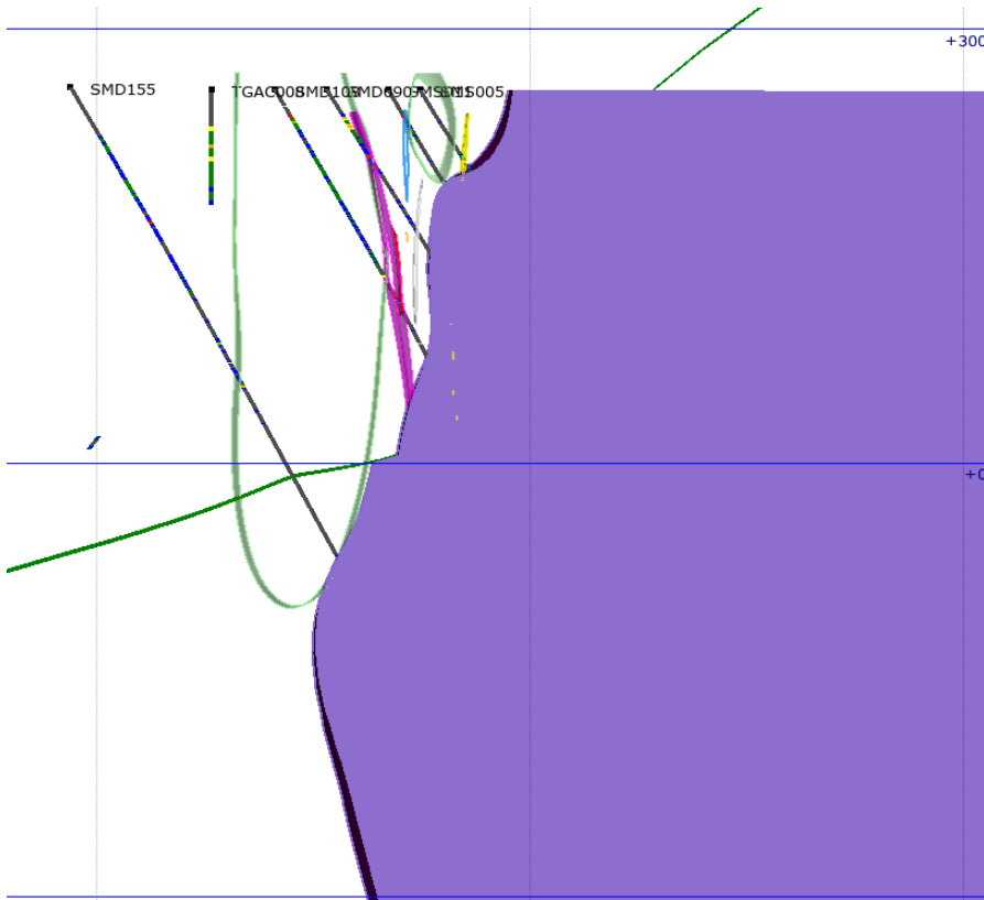
Figure 8a section 4 in figure 3 wide angle view showing a steep NE dipping Cayley Lode, developed only above the LAS, in an area where only a small embayment in the ultramafic hosts one of two granodiorite bodies.
