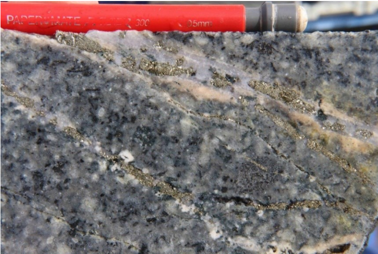
Photo 20 Toora West diorite porphyry cut by quartz-pyrite-chalcopyrite vein with albite selvage, STMD6, 56.8m.
