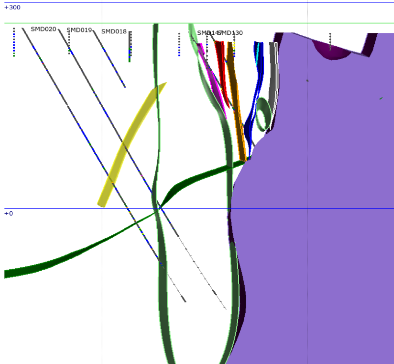
Figure 6 section 2 in figure 3 shows a negative flower structure array of a series of Cayley Lodes developed in a dilatant embayment in the Staveley Volcanics-ultramafic contact.
