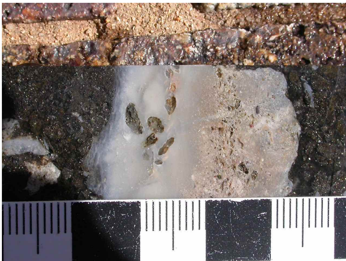
Fig. 7: Offcut from the polished thin section showing a large chalcedonic quartz fragment with faint colloform banding and scattered cavities. The dark material on either side contains scattered small fragments of clay-rich altered rock, disseminated chromite and fine grained sulphides.
