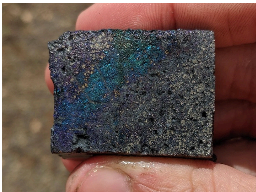
Fig. 1: Drill core sample of semi-massive sulphides, with bornite-dominant domain at left and more pyrite-rich zones either side. There is considerable gangue quartz, hosting scattered small cavities.
