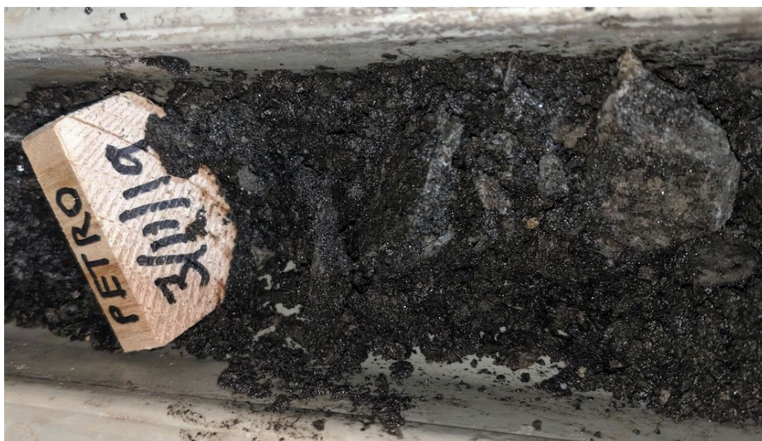
Fig. 6: Drill core sample of strongly fragmented material. Large fragments are dominated by fine grained chalcedonic quartz. Dark colour is due to sulphide-impregnated clay and disseminated chromite.
