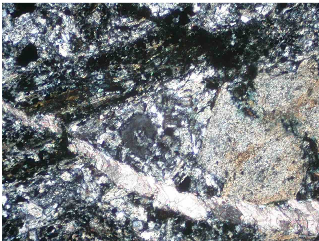
Fig. 12: Altered porphyritic microdiorite showing an albitised plagioclase phenocryst at right and a pseudomorph after a former hornblende phenocryst at left, replaced largely by chlorite (dark). The groundmass contains albite, chlorite and minor quartz and apatite, with the rock
