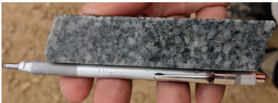
Fig. 38: Drill core sample of strongly porphyritic dacite, characterised by abundant plagioclase phenocrysts in a fine grained grey quartzofeldspathic groundmass. The rock has moderate alteration to chlorite, albite, sericite and a little anhydrite, carbonate and trace chalcopyrite.
