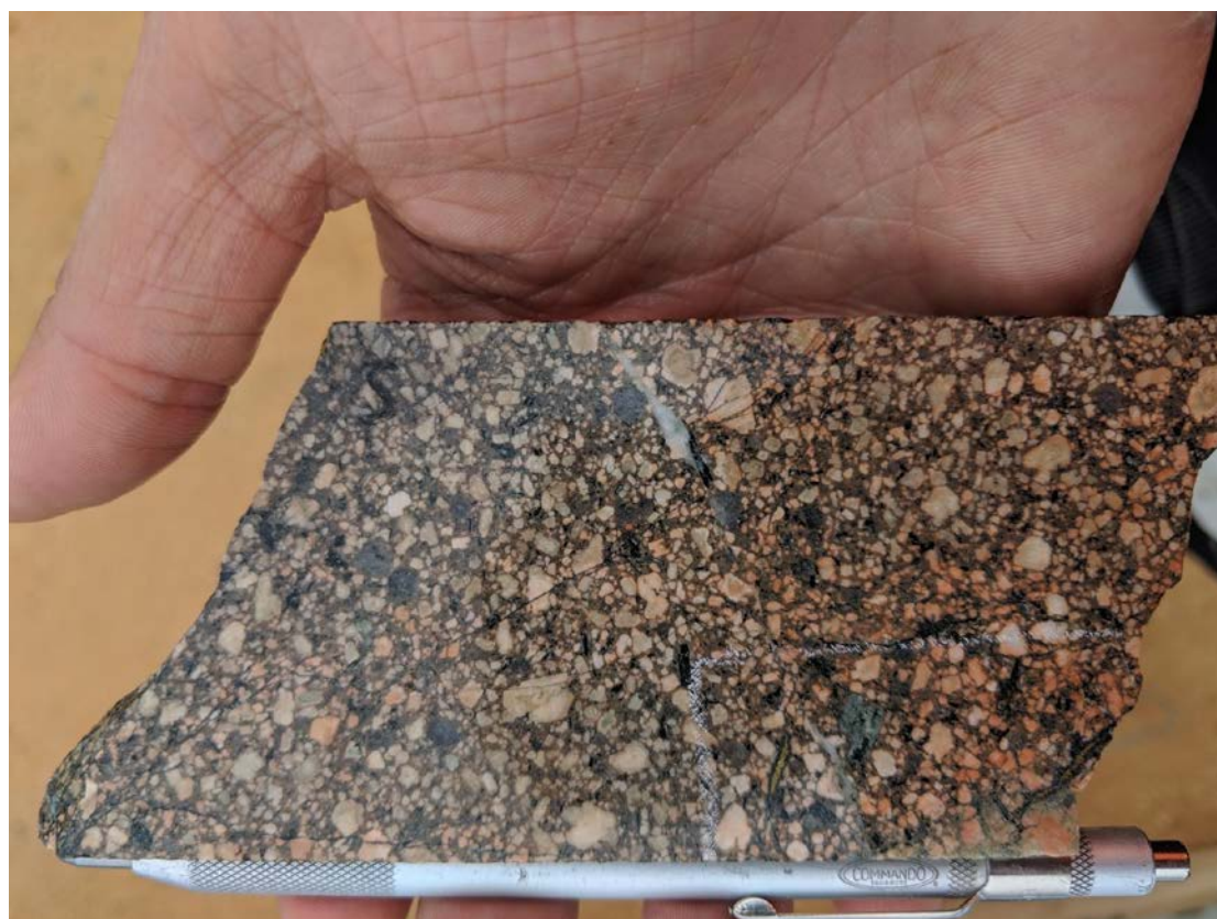
Fig. 1: Drill core sample of altered, strongly porphyritic dacite. Pinker zone at right has stronger K-feldspar alteration.
