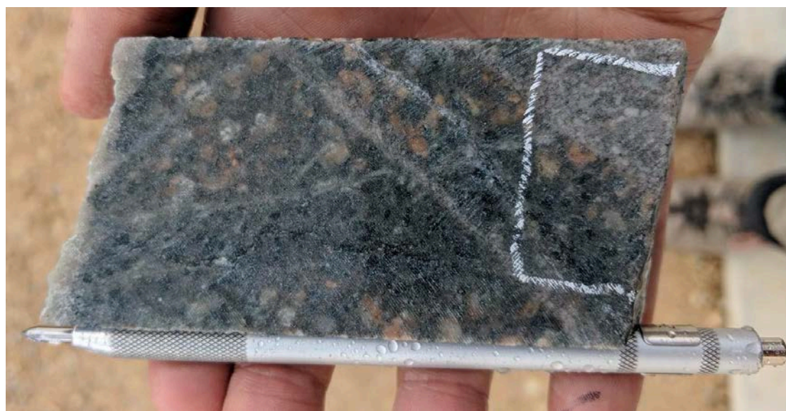
Fig. 47: Drill core sample of moderately to strongly altered porphyritic dacite containing scattered pink to creamy, partly replaced plagioclase phenocrysts, and with dark grey-green colour due to chlorite alteration. At upper right is a small zone of intrusive, medium grained leucotonalite.
