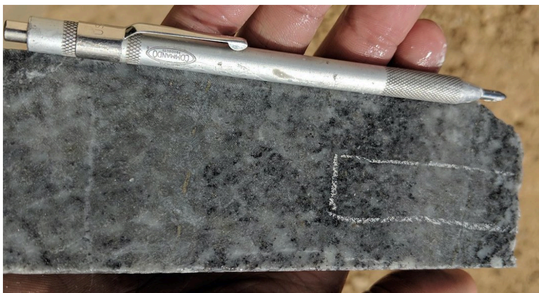
Fig. 44: Drill core sample of strongly phyllic altered porphyritic felsic igneous rock (e.g. microgranodiorite or microtonalite). It formerly contained phenocrysts of plagioclase, ferromagnesian material and uncommon quartz. Alteration of quartz-sericite (-pyrite) type was imposed. Small dark grey zones contain pyrite and trace bornite.
