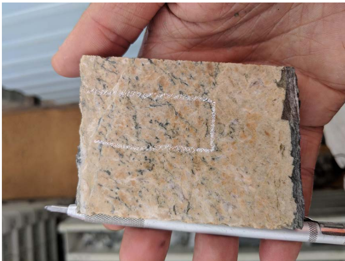
Fig. 17: Drill core sample of strongly altered porphyritic dacite, with an alteration assemblage of albite, calcite, quartz and sericite. The small grey disseminated aggregates are fine grained chalcopyrite. At right is a grey calcite vein containing a little disseminated pyrite.
