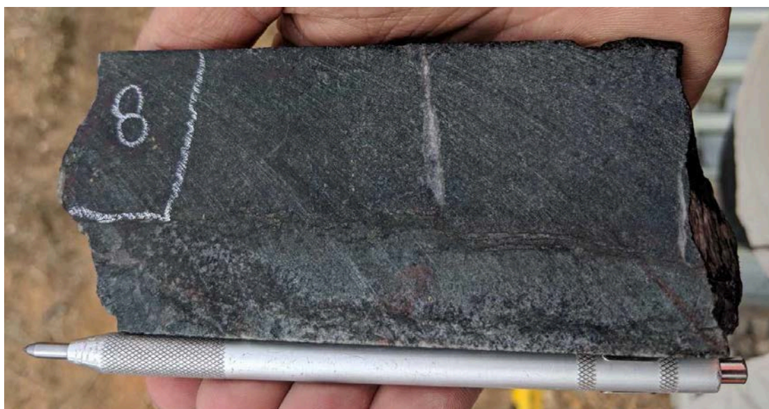
Fig. 24: Drill core sample of intensely altered mafic to ultramafic rock, with dominant replacement assemblage of chlorite and quartz, plus minor anhydrite and hematite. Paler grey zone tends to contain more abundant anhydrite, along with gypsum, clay (dickite), chlorite and quartz.
