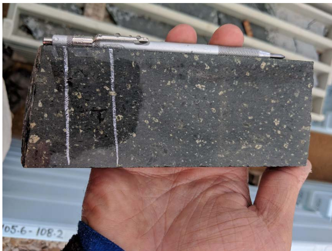
Fig. 14: Drill core sample of massive porphyritic microdiorite, with altered plagioclase phenocrysts, a few hornblende phenocrysts, and a fine to medium grained groundmass. The rock has pervasive development of albite and chlorite, with minor epidote, carbonate and quartz.
