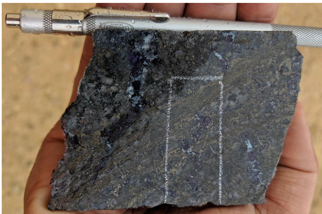
Fig. 29: Drill core sample of intensely altered rock, possibly of felsic porphyritic type, showing replacement by abundant quartz and pyrite, and at left, by dark veinlike masses of bornite and chalcocite.
